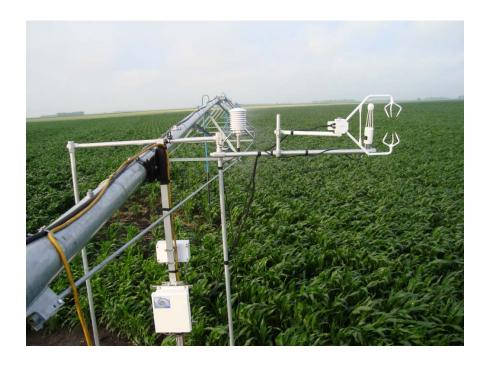
Figure 1. Eddy covariance system measuring CO<sub>2</sub> and H<sub>2</sub>O fluxes above an irrigated corn field.
